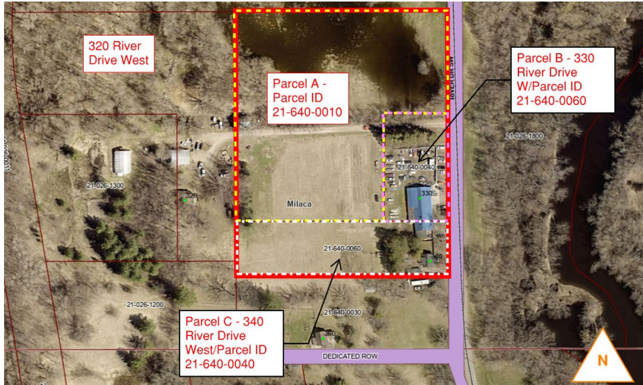
Figure 1: Aerial of the site, per Mille Lacs County GIS. The subdivision area is outlined in red, with the individual parcels outlined in dashed lines. Road right-of-way is shown in purple, other parcel lines are shown in red.
